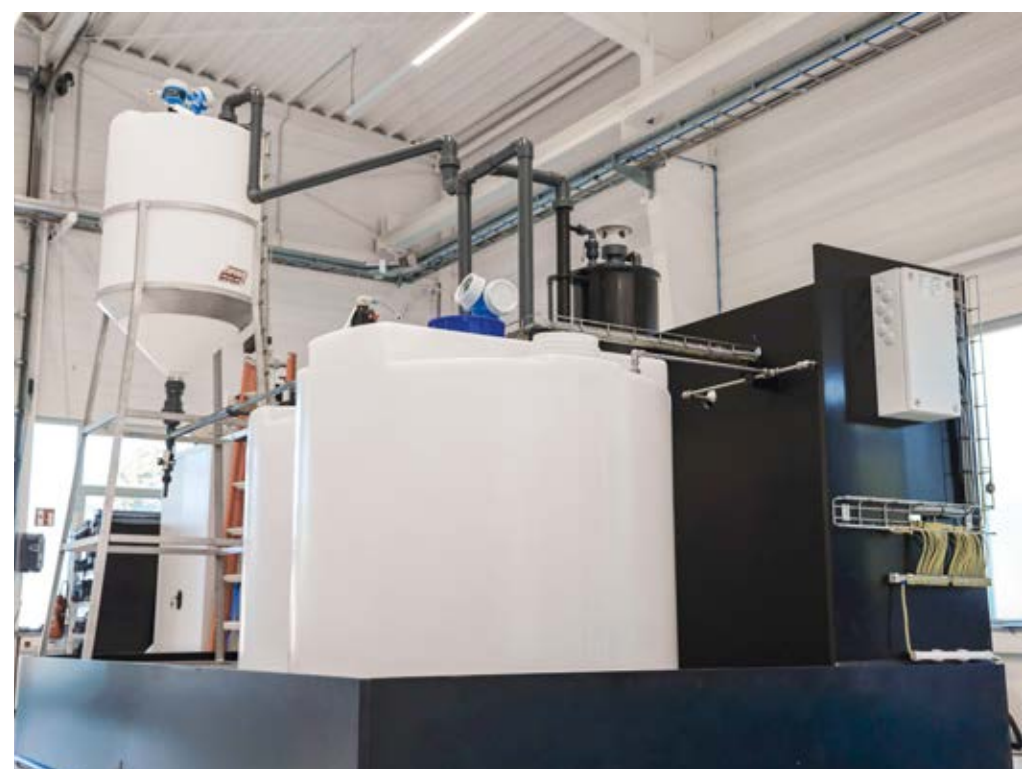
Dilution station for ammonia with storage tanks: dilution of 25% ammonia to 0.5 to 2% ammonia and storage in two storage tanks.
