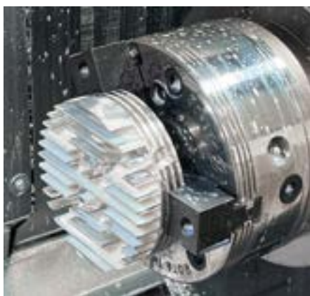
Fully machined H2 cylinder head
