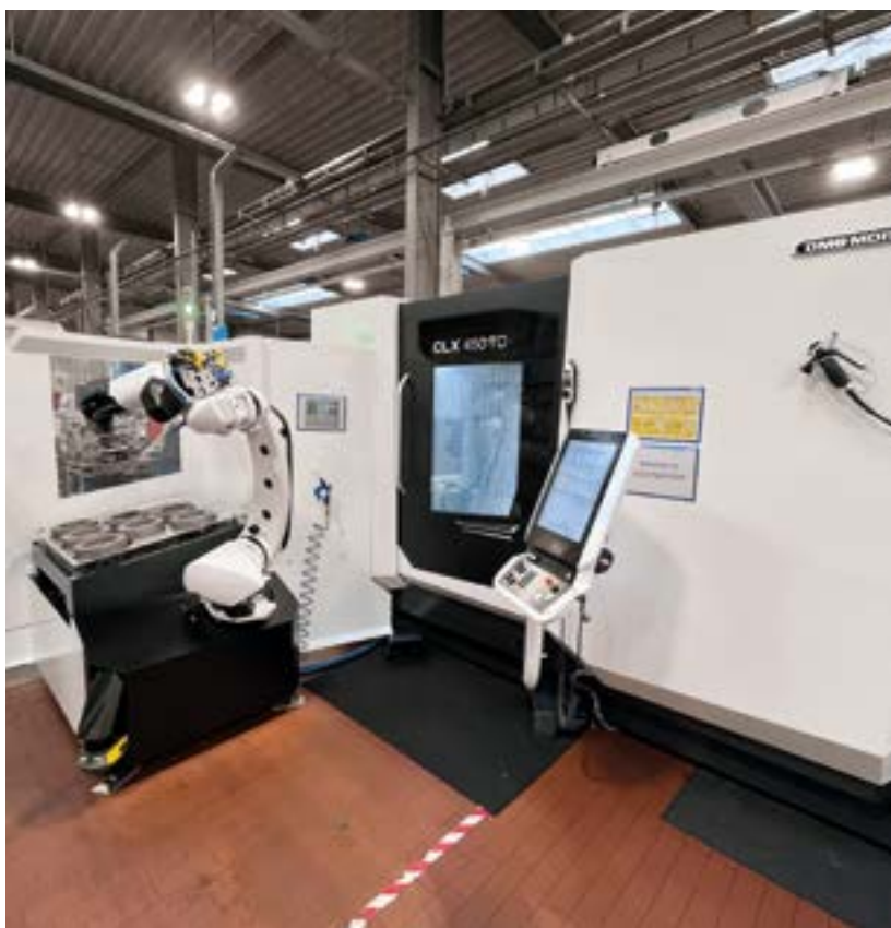
DMG MORI CLX 450 TC in combination with the Robo2Go system
