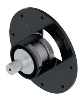
The assembly of the bearing box in the pump casing guarantees perfect alignment, as well as complete absorption of the forces on the shaft. The bearing box supports the reinforced and oversized bearings and the pump shaft, enabling a compact and very robust design. This guarantees unbeatable robustness and power of the pump, even under the most difficult conditions in continuous operation with pressures up to 10 bar. Minimal maintenance costs and downtime.
