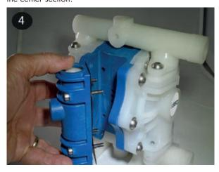
First hand tighten only each cap screw (item 1) until the cap screw head makes contact with the valve body. Torque the cap screws in an "X" pattern. Do not exceed 15 in-lbs (1,7 Nm).
