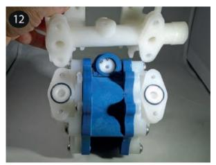
Stand the pump upright onto the suction manifold feet (item 12). Place the valve balls (item 15), valve seats (item 14), and seat o-rings (item 13) into the discharge manifold (item 16) in the same order as the suction side was done in step 11. Place the discharge manifold atop the pump, tighten, and torque the discharge manifold bolts (item 11) in an "X" pattern. Torque to 50 in-lbs (5,6 Nm).
