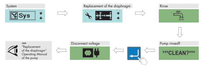
The counters for diaphragm operating hours and diaphragm service life are reset after successful diaphragm replacement.
