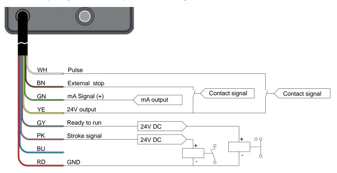
Connection of a pulse signal with External Stop (external control voltage / PLC):
