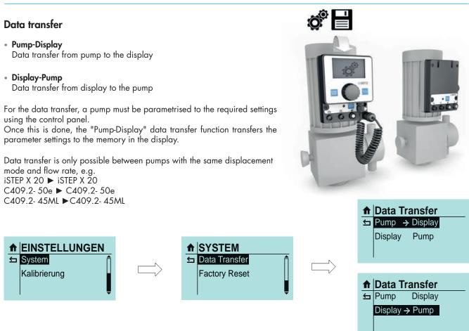
The display can now be unscrewed from the pump and connected to another pump. Using "Display-Pump" data transfer, the parameters stored on the display can be transferred to the second pump. This process can be repeated any number of times with other pumps. After the data transfer calibrate the pump(s).
