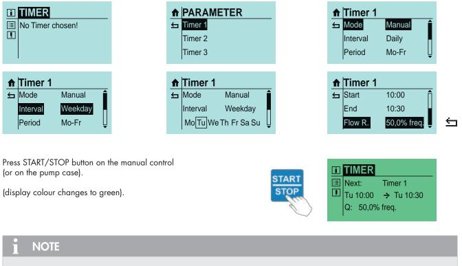
Any possible overlapping of specified time periods is prevented (an appropriate message is shown on the display).
