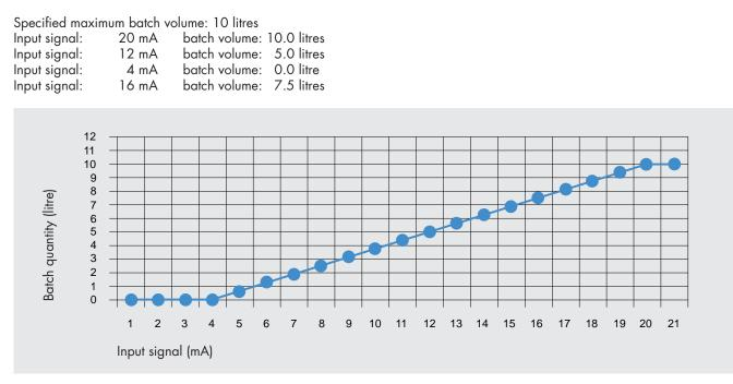
The stroke speed is set in the same way as for the batch quantity. First select the maximum value that corresponds to the 20 mA signal. The delivery rate can now be set using an appropriate input signal between 4 mA and 20 mA.
