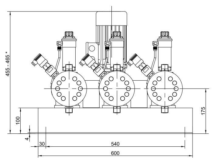
\* at 409.2-1,6e to -25e: 455 mm at 409.2-50e to -350e: 465 mm
